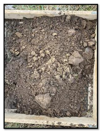
Figure 53: General test pit fill showing sandy clay soil with light brown subsoil (MH1059-D148).
