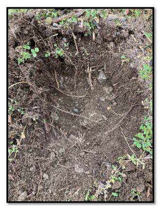
Figure 55: Excavated test pit on the top of the rise in the central eastern portion, gravel on bedrock (MH1059-D197).
