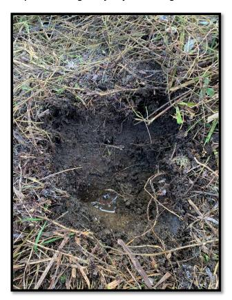
Figure 54: Standing water in the bottom of test pit at the edge of the marshy area (MH1059-D178).
